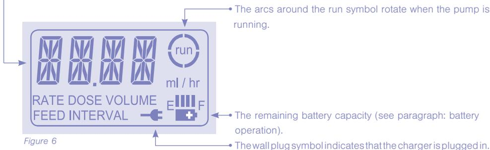
The back light of the display turns off 10 seconds after the last key is pressed.
